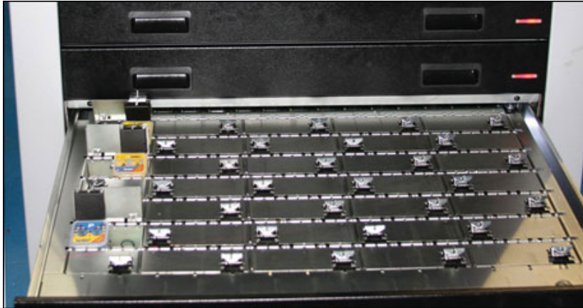
Iscar's Matrix tool management system combines the automated tool dispenser with management software to control inventory, streamline purchasing, and drive down costs.
