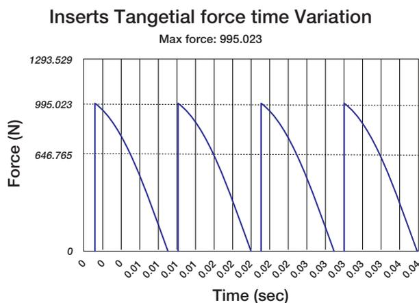
**Fig. 34.** Graph depicting the variation of tangential cutting force during milling a square shoulder
