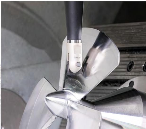
**Fig. 5. Machining the complex surfaces of a propeller with a barrel-shape endmill.**
