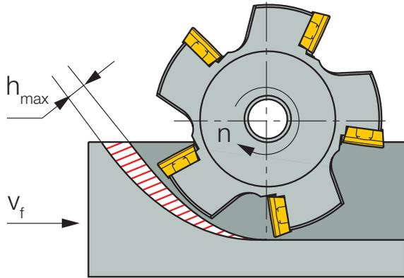
Fig. 10. Up (up-cut or conventional) milling.
