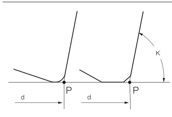
Fig. 19. The cutting diameter ( $d$ ) in accordance with ISO 6462 standard.
