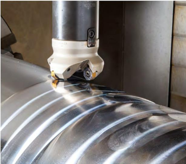
**Fig. 44.** Turn-milling is an effective method in rough machining heavy rotary parts.
