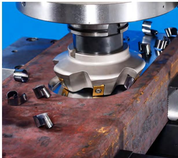
**Fig. 51. Wet cooling is not recommended for heavy-duty milling of steel with indexable tools.**
