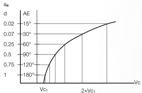
Fig. 38. Cutting speed as a function of radial engagement.
