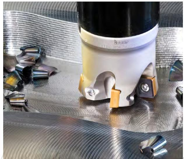
**Fig. 41. A versatile indexable high feed milling tool is suitable for productive rough machining open planes, 3D surfaces, pockets, and cavities.**
