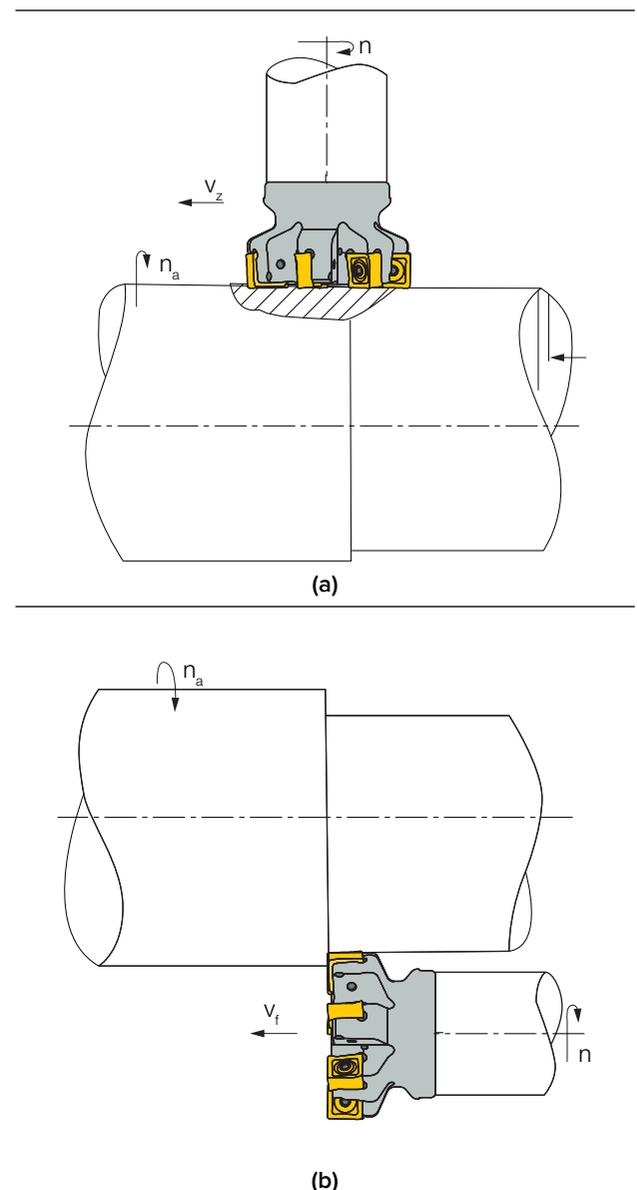
Fig. 43. Peripheral (a) and face (b) turn-milling operations.
