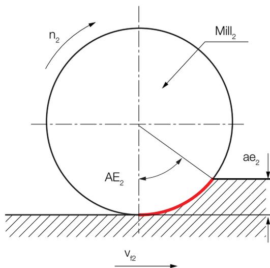
Fig. 26. Contact arc, angle of engagement AE, and width of cut (radial depth of cut)  $a_e$ .
