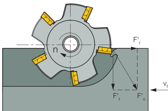
Fig. 33. Force diagram in down (climb) milling
