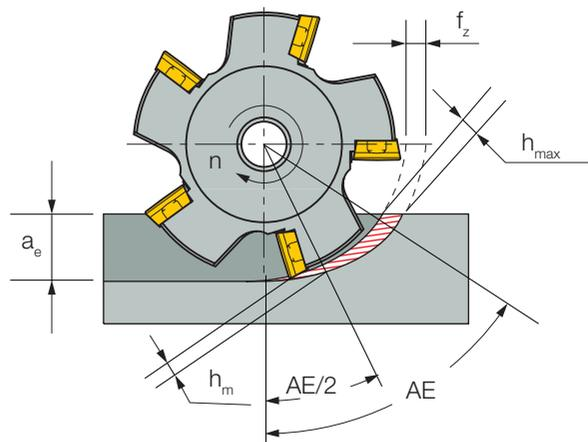
Fig. 27. Chip thickness as the function of a width of cut (radial depth of cut)  $a_e$ .
