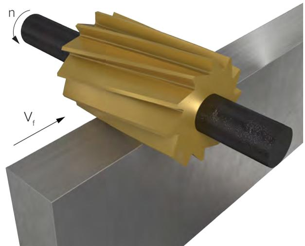
Fig. 2. Peripheral (slab) milling.
