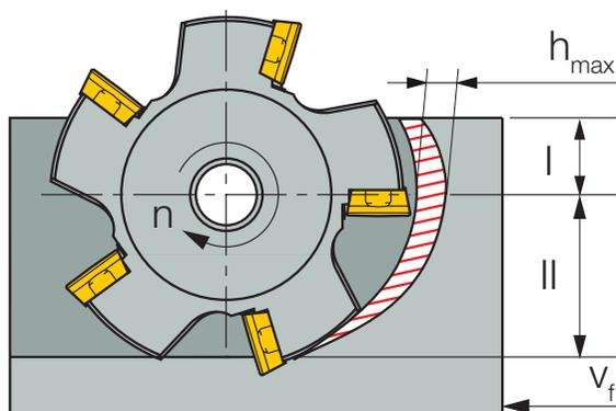
Fig. 12. Combination of up and down milling when the axis of the tool lies within the material being machined. Area I features up milling, while area II is characterized by down milling.
