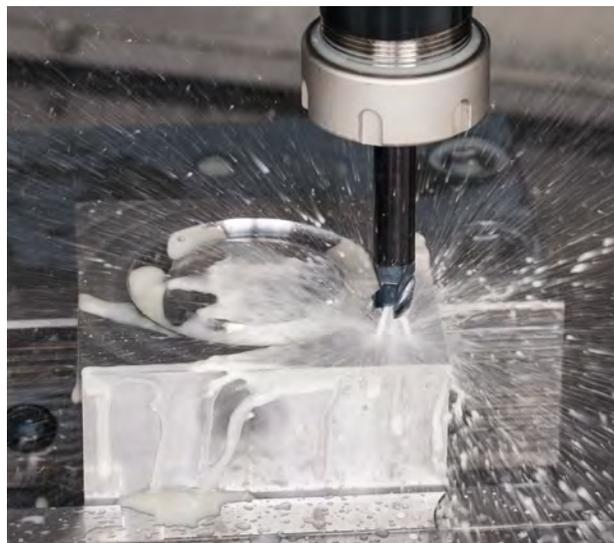
**Fig. 50.** A pinpointed high-pressure coolant jet significantly improves performance of a MULTI-MASTER endmill when machining hard-to-cut aerospace materials
