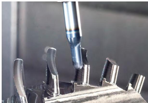
**Fig. 39.** Trochoidal milling is an effective method for improving productivity during the rough machining of geometrically complex surfaces.
