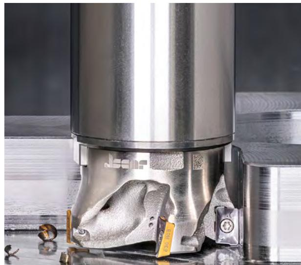
**Fig. 37. A shell-mill with a titanium body harnesses the advantages of additive manufacturing (AM) technology.**
