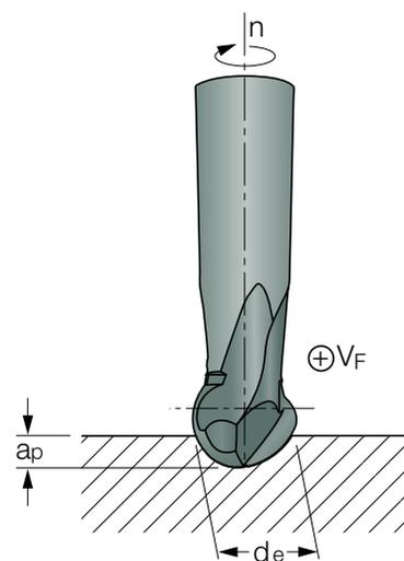
Fig. 23. The effective diameter  $d_e$  of a ball-nose endmill.
