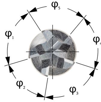
Fig. 20. A solid carbide endmill with differential pitch features unequal teeth spacing, as shown from on-end view.
