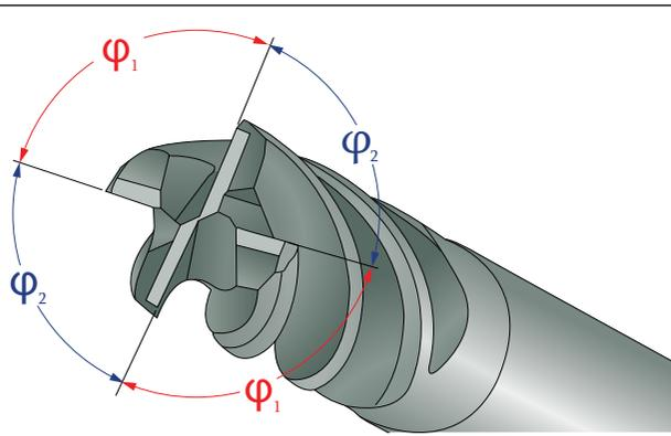
**Fig. 21. A solid carbide endmill with alternating teeth spacing has each pair of pitches being identical.**
