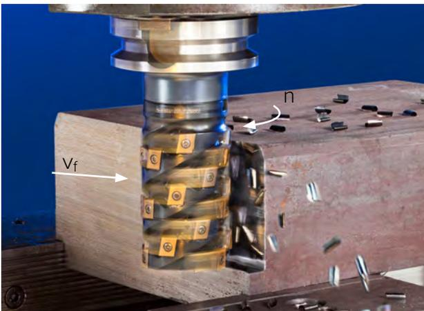
Fig. 1. Example of motions in milling: primary motion is the rotation of a milling cutter with rotational velocity  $n$ , while feed motion involves the rectilinear movement of a machine table carrying a workpiece mounted on it, with a linear speed  $v_f$ .
