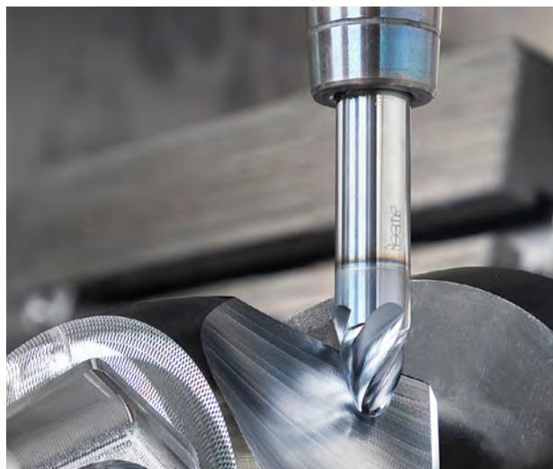
Fig. 46. Precise solid carbide endmills enable accurate milling of complex 3D shapes.
