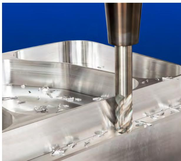
Fig. 4. Milling shouldered surface by solid carbide endmill.
