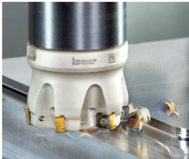
Fig. 45. Indexable milling cutters feature various insert shapes and a wide diameter range.
