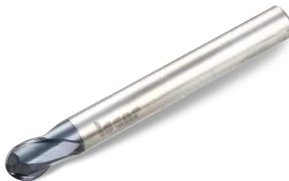
Fig. 14. A solid carbide ball nose endmill. (The ball-nose shape of this specific profile end mill makes it perfect for machining 3D surfaces, especially in semi-finish to finish operations. It is designed with a shank-type structure and produced from tungsten carbide).
