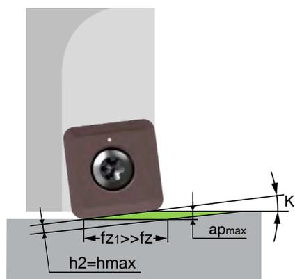
Fig. 40. Geometrical relations between feed per tooth, cutting edge angle, and chip thickness.
