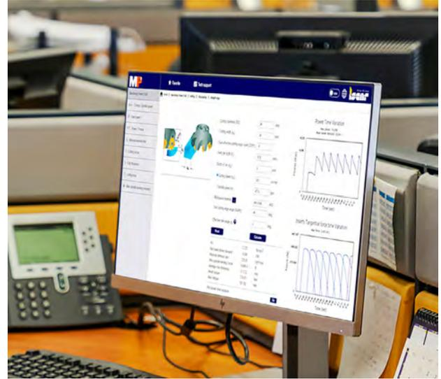
Fig. 31. ISCAR’s Machining Power Calculator is an effective tool for accurate online calculating of cutting power and cutting forces in milling applications.
