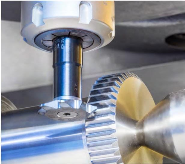
**Fig. 48.** The application range of T-SLOT extends beyond milling slots and grooves. This concept has also been utilized in the milling of threads, gears, and splines. Furthermore, the T-FACE family has adopted this concept for use in face milling applications.
