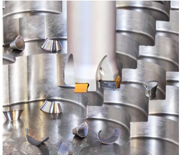
**Fig. 42. Plunge-in milling enables productive rough machining to pre-shape complex 3D surfaces.**
