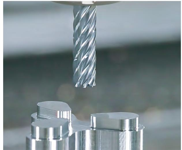
**Fig. 38.** ISCAR's 7 flute solid carbide endmill, intended for HSM, features different helix angles, variable pitch, and chip-splitting grooves on the cutting edges.
