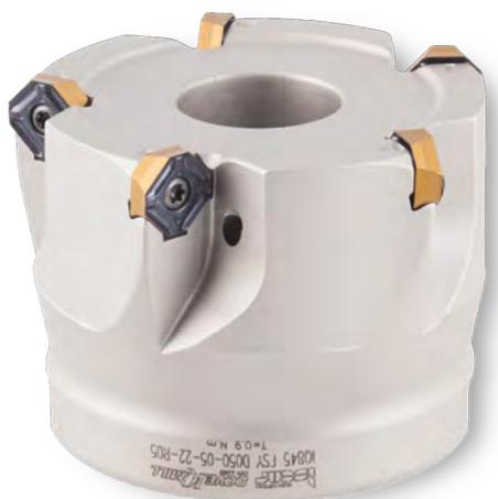
Fig. 13. An assembled right-hand face mill with indexable inserts. (This general-duty mill is primarily used for machining open planes. It features a shell-mill configuration and is equipped with indexable carbide inserts).
