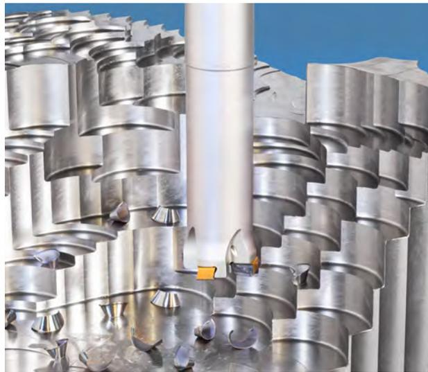
**Fig. 7. Machining a workpiece by plunge milling**
