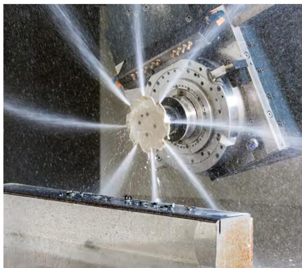
**Fig. 52. ISCAR's TANGSLIT indexable slitting cutters with inner coolant channels directed to each and every cutting edge is suitable for use with both standard coolant and high-pressure coolant applications.**
