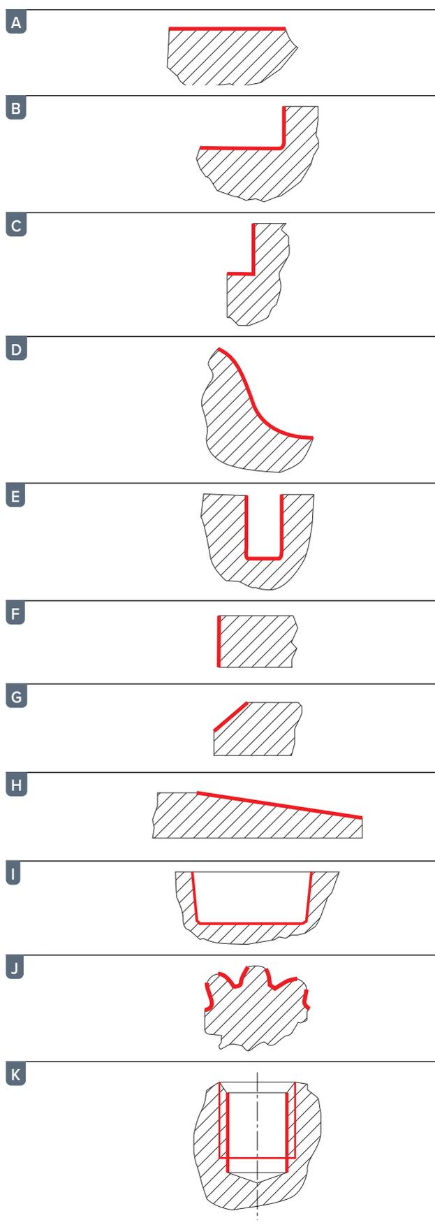
Fig. 9. Illustration of surfaces machined using primary milling operations.
