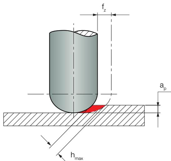
Fig. 25. Axial chip thinning in milling with a ball nose milling cutter.
