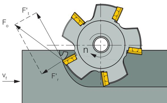
Fig. 32. Force diagram in up (conventional) milling.
