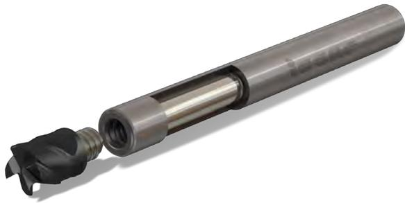
**Fig. 35.** The anti-vibration shank for mounting exchangeable **MULTI-MASTER** heads incorporates the concept of an internal absorber.
