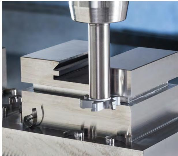
**Fig. 6. Milling slot by side-and-face milling cutter.**
