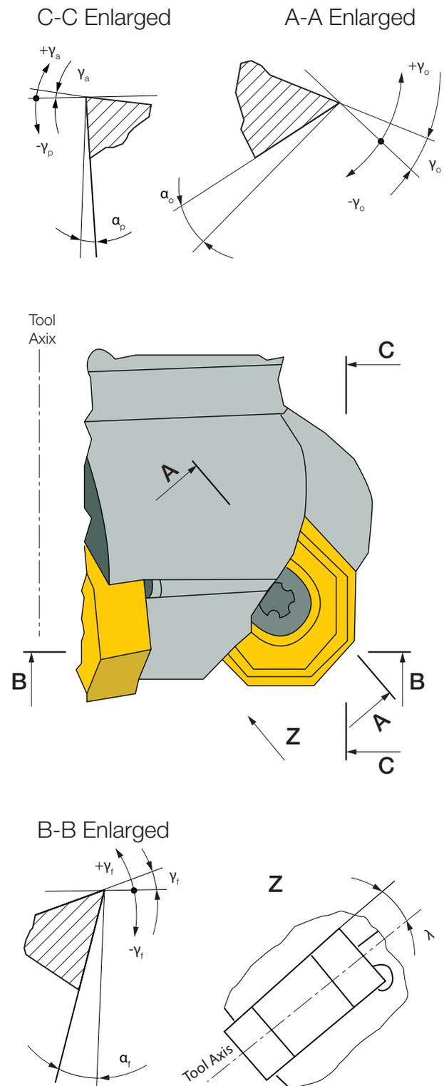
Fig. 17. The rake  $\gamma$  and the clearance  $\alpha$  of the indexable milling cutter shown in Fig. 15, each measured in different reference planes.
