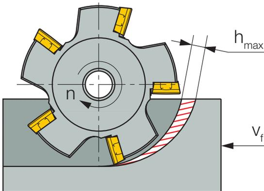
Fig. 11. Down (down-cut or climb) milling.
