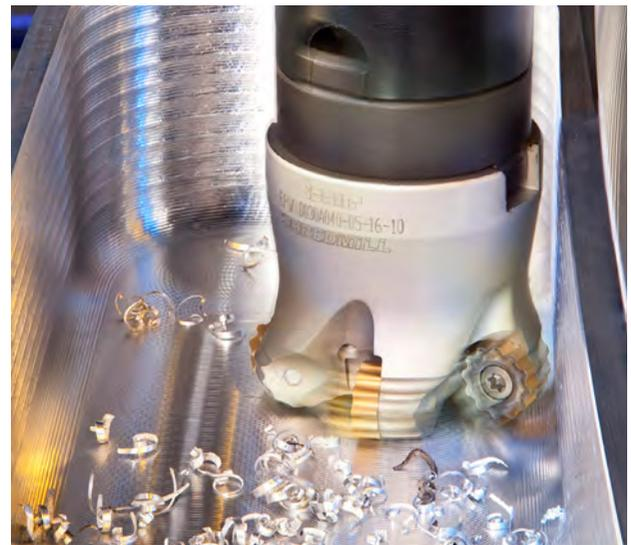
**Fig. 36.** Chip-splitting cutting geometry can greatly contribute to the stability of milling operations in unfavorable conditions.
