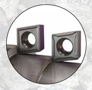
The latest rake face designs F3M and F3P for ISO standard turning inserts are intended specifically for hard-to-machine austenitic stainless steel and superalloys. Their positive rake-angle geometry reduces the cutting force and ensures smooth cutting action, while the set of deflectors on the rake face improves chip control.
