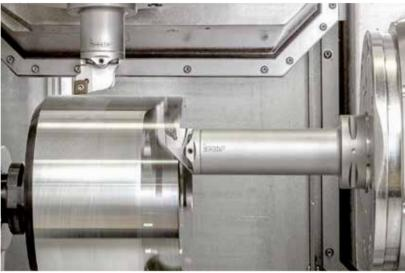
What else can be new in ER spring collets? Tool manufacturers have developed a rich variety of precise collets that offer coolant supply capability. For example, ISCAR's new updated ER rubber sealed collets with an extremely narrow collapse range ensure better clamping force, maintain high runout accuracy of 0.005 mm (.0002"), and facilitate 4 cooling jets.
