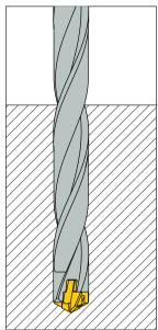
• Prior to using 8xD or 12xD drills, it is recommended to drill a 0.5xD pre-hole using a short or centering drill. Enter the pre-hole at slow speed and feed until .08-.20" from its bottom. Start the cooling system and increase rotation to recommended drilling speed. Hold for 2-3 seconds, then, continue at the recommended drilling feed.
