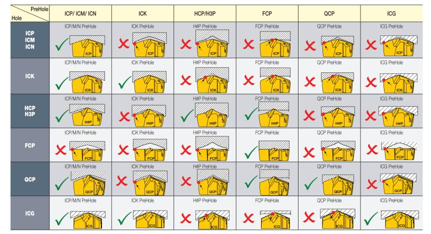
\*For proper insert performance and centering, a bigger insert within a .039" range of the same diameter may be used
