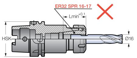
Important: Never insert the collet parallel to the extractor ring. Doing this will chip or break the extractor's teeth. When unclamping the nut, the collet will self-release from the chuck by means of extractor teeth.
