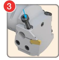
The tool is supplied with a long upper clamping screw which is inserted diagonally, two short bottom clamping screws, two middle (securing/sealing) screws and four sealing O-rings (two are spare).
