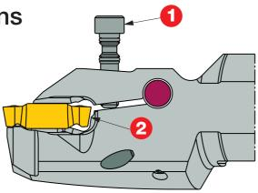
1. Position the insert in the pocket so the notch on the insert sits on top of the frontal bulge of the pocket
