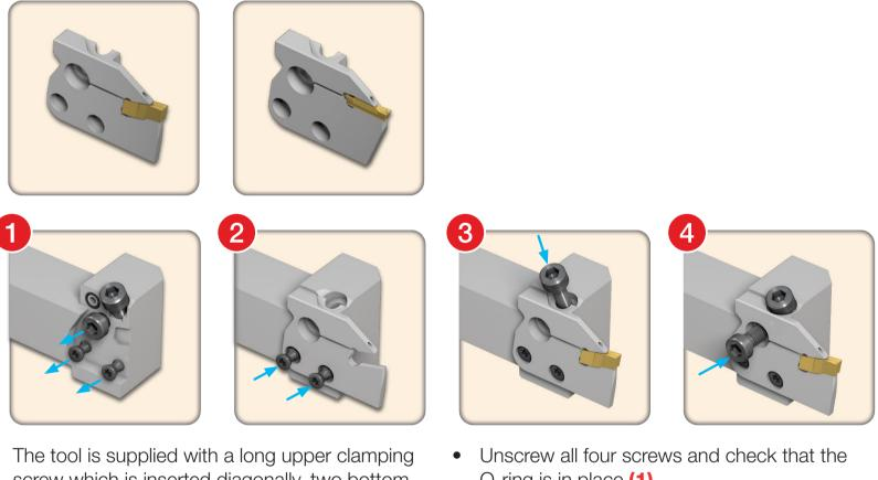
screw which is inserted diagonally, two bottom clamping short screws, one middle (securing) screw and three sealing O-rings (two are spare).
