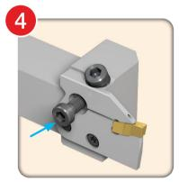
The tool is supplied with a long upper clamping screw which is inserted diagonally, two bottom clamping short screws, one middle (securing) screw and three sealing O-rings (two are spare).
