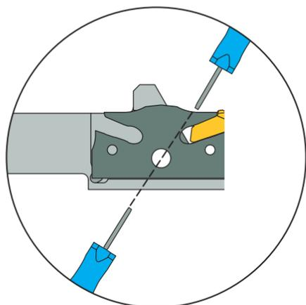
The key can be inserted from both sides.
