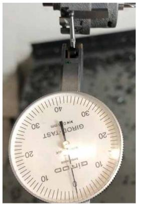
Use a dial indicator to align the spindle housing on the ground edge
