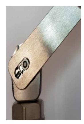
2 Lock the shaft using the dedicated key as shown in the picture, and screw the collet in position
