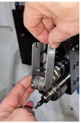
Insert the cutting tool into the collet then tighten the collet using both keys as shown in the picture
