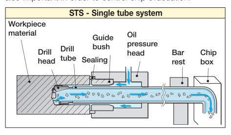
Flow chart of coolant in deep hole drilling
