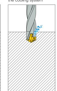
**4** Continue drilling at recommended cutting conditions
