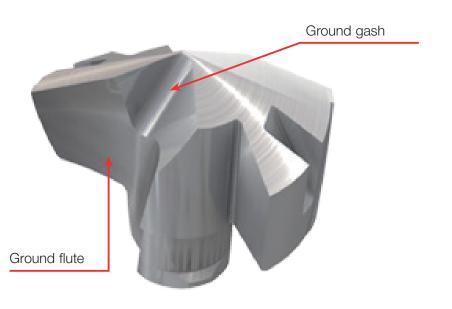
The drill head has ground flutes for smooth, uninterrupted chip flow and a ground gash for improved penetration.
