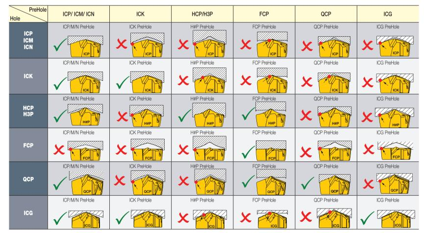
\*For proper insert performance and centering, a bigger insert within a 1.0 mm range of the same diameter may be used
